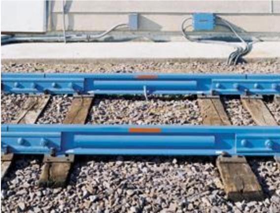
Trade scale – it truly is a weight estimator. It is my customers experience that this device will provide a weight estimate that is within 8 to 10% of the actual weight. This customer uses the Weighline Railscale weight information to fill the railcars with the product. The Railcar then is transferred to the Certified MettlerToledo Railscale – that is accurate!
